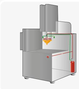
FIRETRACE INDIRECT SYSTEMS ARE AVAILABLE WITH AN OPTIONAL MANUAL RELEASE, ENABLING AN OPERATOR TO ACTIVATE THE SYSTEM AT THE FIRST SIGN OF TROUBLE.
