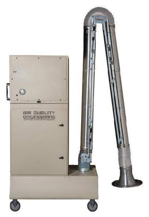
The M66 from Air Quality Engineering, Inc. is a self-contained media air cleaning system designed for use in source capture applications where mobility is desired. The M66 can be ordered in a three-stage filtration configuration which will effectively remove a broad range of airborne contaminants including fine dust, smoke, soot, vapors, mist, VOC's and more at a rate of up to 2000 CFM.
